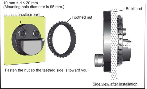
6. See the figure below to insert the nut lock all the way in to prevent the toothed nut from loosening.
